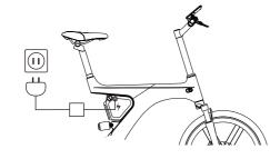
Charge the battery while it is still in the e-bike with the provided charger.
