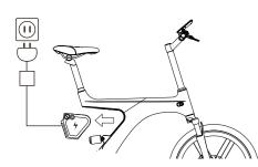
Remove the battery and charge it with the provided charger.
